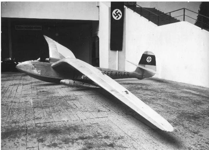
rudder, coupled to the main rudder, was fixed below the fuselage and proved to be very effective at low speeds up to 15 to 20 km/h. The underside of the fuselage was covered with a heavy cloth, fixed with adhesive and painted with multiple layers of dope.
