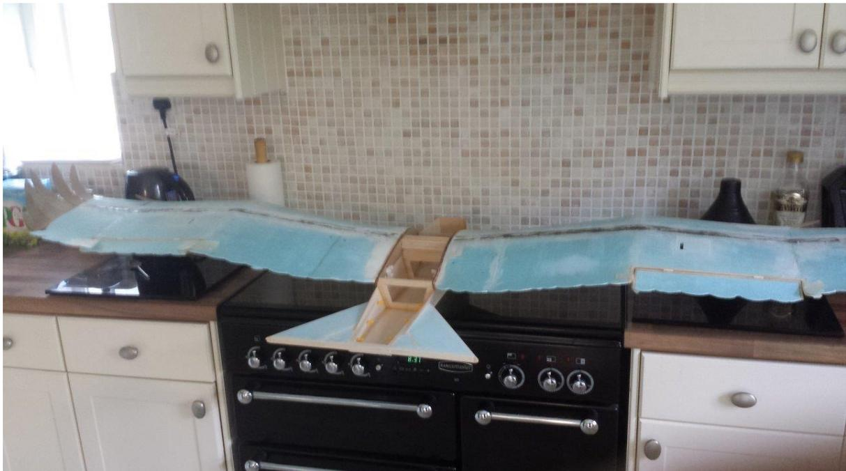
To connect the wings to the body 2 nylon bolts were added to each of the wing roots in preference to the designer's elastic bands and hooks. Makes for a nice tight fit and the bolts can be replaced quite easily if one breaks. I wanted easy access to Eddie's insides so a front, middle and rear hatches were added and shaped to match the profile of the neck and shoulders. All held in place by rare earth magnets, another departure from the original plan.
